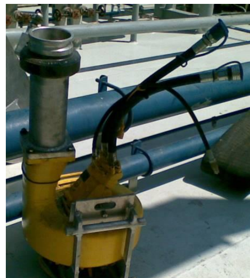
Figure 6 Marflex Centrifugal Pump MSP150
