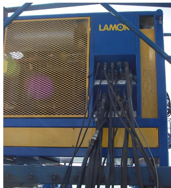
Figure 12 Power-pack hydraulic connections
