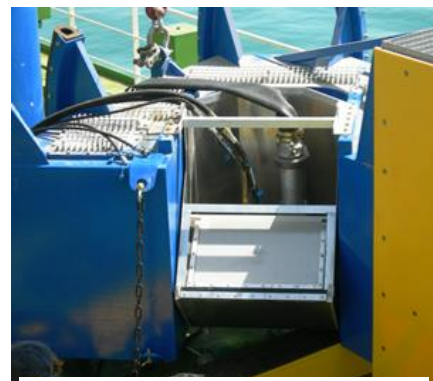
Figure 5 Weir Skimmer module
