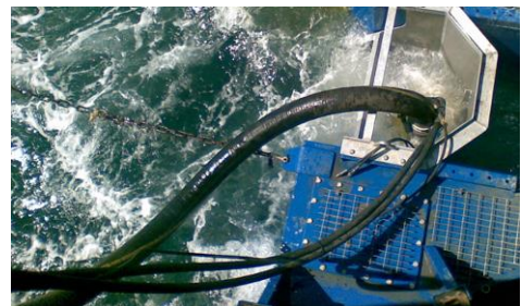
Figure 10 Oil transfer hose connected to the weir module
